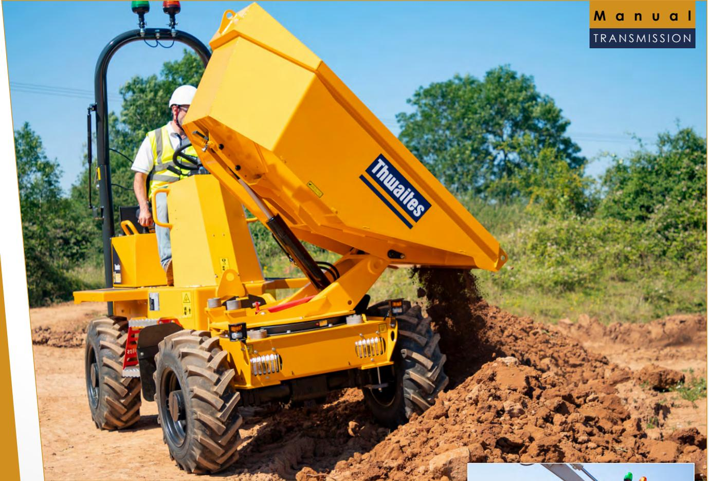
The Thwaites 2 Tonne Power Swivel, Stage V dumper is manufactured with contractors and hirers in mind – ensuring operator safety, reducing risk on site and improving performance. Powered by an 18.1 kW 3-cylinder Yanmar engine, delivering 107 Nm max torque for optimum traction and control. This machine is driven by a Manual transmission.
