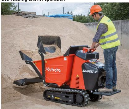
The models KC70SL-4 and KC70VSL-4 are crawler dumpers featuring a self-loading shovel. This device is very useful when you need to remove loose material (such as sand or gravel) or to clear demolition rubble. The minimum width of 758 mm allows easy access inside buildings. On the VSL version, the variable undercarriage insures good stability regardless of ground condition. The loading capacity of 700 kg makes the KC70-4 SL/VSL the ideal work mate for moving material on the job site.
