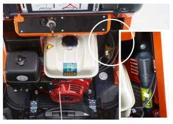
Waterproof document holder for user manuals protected in the locked engine compartment. This allows the operator to have the machine's documents always available.
