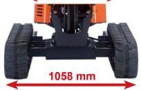
The variable undercarriage extends the overall width from 758 mm to 1058 mm. At minimum width, the KC70-4 can easily go through a standard door. At maximum width, the KC70-4 offers great stability in all conditions.
