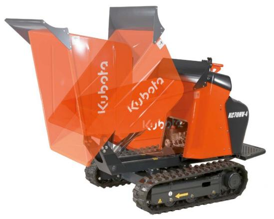
Unloading operation is fast and easy. The profile of the skip has been designed to ensure a quick discharge of the material. With a dumping angle of 88° (85° for HD/VHD versions), all materials exit easily from the skip in any work situation.
