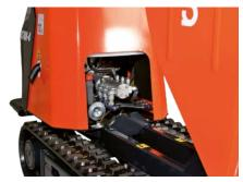
The KC70-4 crawler dumpers are equipped with an hydraulic transmission. This advanced transmission offers smooth control, the operator can select the speed best suited for the terrain, and can easily shift from 3.3 km/h high speed on flat surfaces, to 2.2 km/h low speed for rougher terrain. This system helps make working more efficient and productive, reducing maintenance and also fuel consumption.
