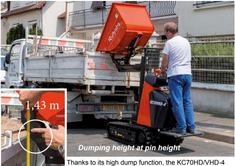
Thanks to its high dump function, the KC70HD/VHD-4 can empty its load up to 1,43m high (pin height). In addition, the dumping reach of 447mm allows easy discharge of the load from the skip, whilst leaving good clearance to the truck edge.
