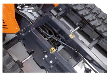
This type of assembly structure reduces the minimum machine width to 758 mm (as standard versions) or can increase width to 1058 mm for extra stability.
